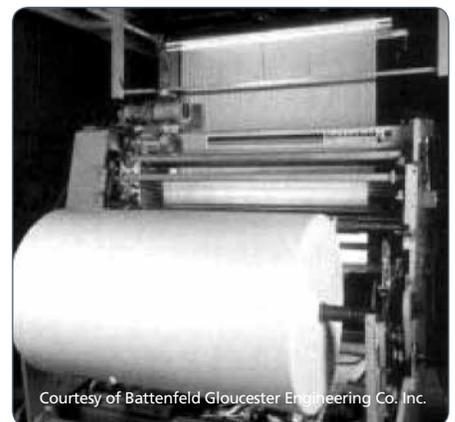
Figure 41: Surface winders have a rotating drum that forces the film roll to turn and, thus, wind up the film web.
