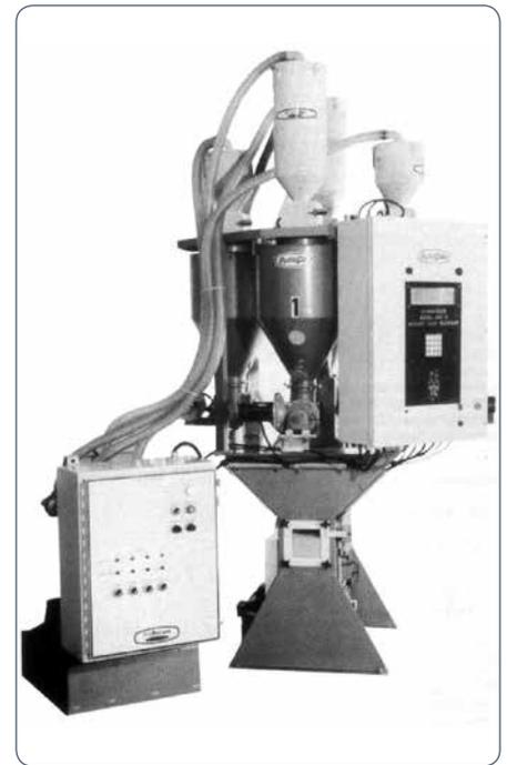
Figure 14: Gravimetric blending units accurately measure components in polyolefin extrusion.
