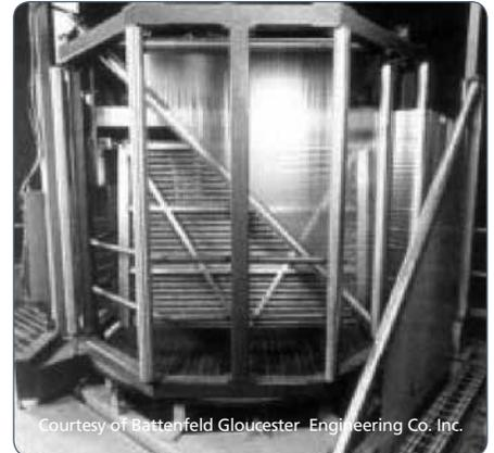
Figure 39: Oscillating (360° or 720°) haul-off units further minimize film gauge variations in the final roll.
