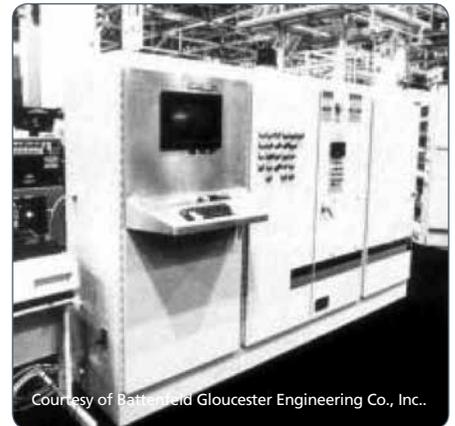
Figure 44: Microprocessor controls handle many film processing variables simultaneously.
