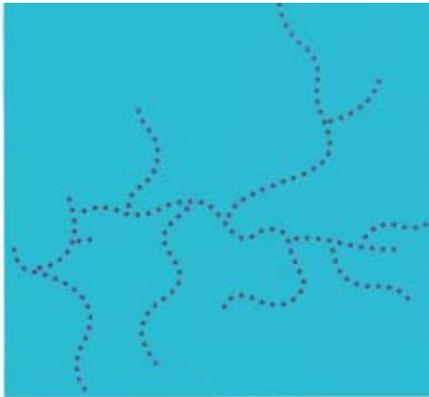
**Figure 3. Polyethylene chain with side branches.**
