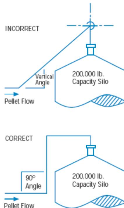
Long radius elbows are not recommended for pellet conveying when streamers are a concern. “Blinded tees,” or other specialty elbows designed to minimize creation of fines and streamers, should be used (**see Figures 6-9**). Contact your LyondellBasell technical service representative for further details.
