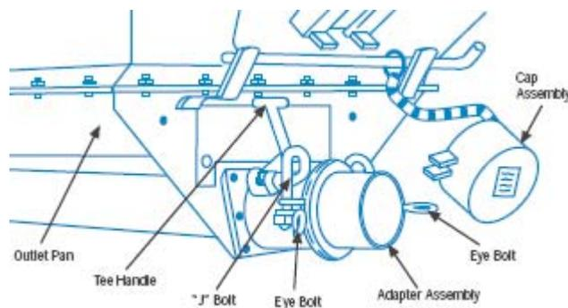
**Figure 13.** Basic components of an adjustable pneumatic outlet.
