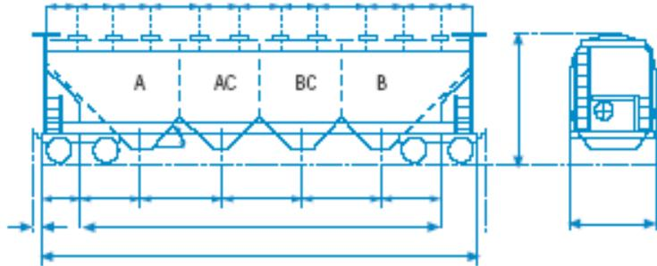
**Figure 2.** A typical hopper car is divided into four compartments.
