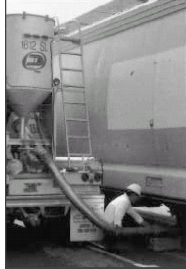
**Figure 15.** A hopper car is unloaded into a hopper truck for shipment to a customer not serviced by a rail line. The truck's air blower is used to unload the car. Note that the conveying pipe does not touch the ground to prevent moisture and contamination from entering the system.
